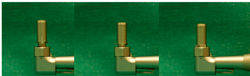
Figure 3 A guide tube directly screwed to the head of the surgical handpiece.
